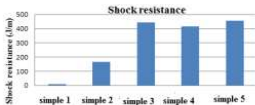
Fig. 2. Impact strength of doubly-reinforced heterocomposite polymer materials based on the ED-20 binder
