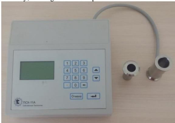
**Fig. 2.5. Surface meter of dispersed materials PSX-11A**
