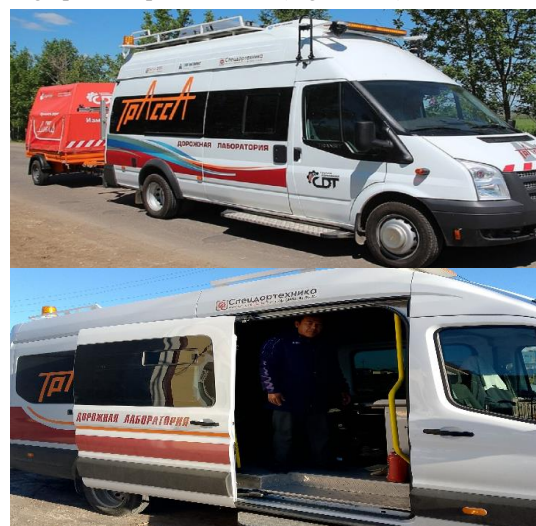
Fig. 1. "TRASSA" mobile road laboratory vehicle
