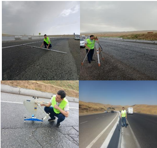
Fig. 1. The process of measuring the longitudinal slope of the road, the width of the roadway, and the flow of vehicles
