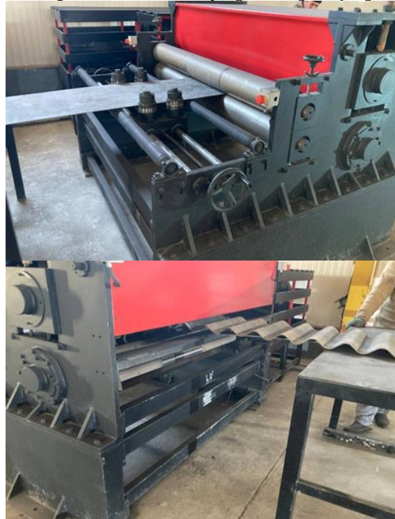
1-rasm. Qo'shtavr devorchasini gofrlash jarayoni (Samarqand)
