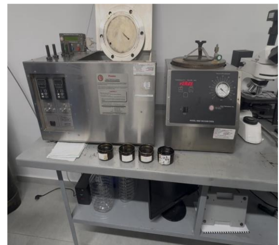
Fig. 1. PAV-aging process of modified bitumens in the laboratory
