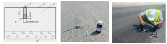
Fig. 2. Scheme for measuring the temperature of asphalt concrete:
