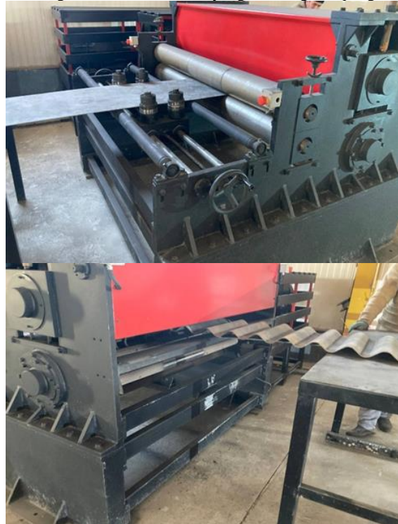
1-rasm. Qo'shtavr devorchasini gofrlash jarayoni (Samarqand)
