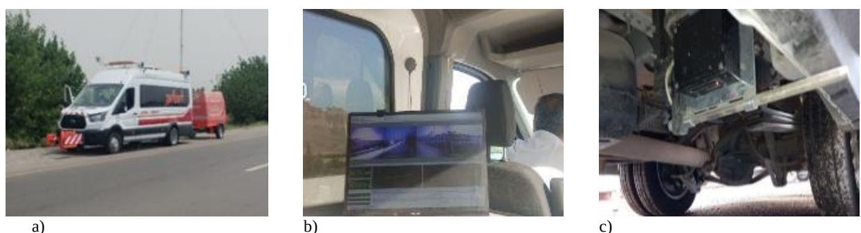
Fig. 2. “TRASSA” mobile road laboratory complex: a) general view; b) operator workstation; c) measuring equipment
