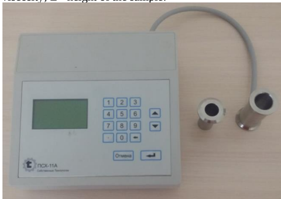
Fig. 2.5. Surface meter of dispersed materials PSX-11A
