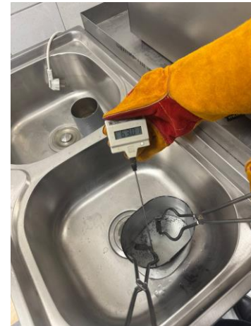
Fig. 2. Monitoring of the quenching medium temperature: thermometer reading of 63.0 °C in the bath with preheated water
