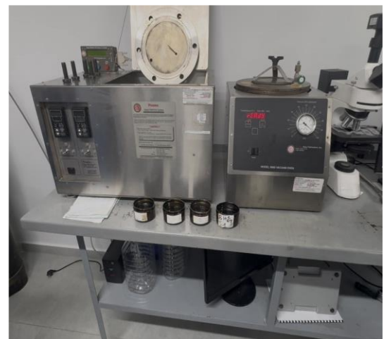
Fig. 1. PAV-aging process of modified bitumens in the laboratory
