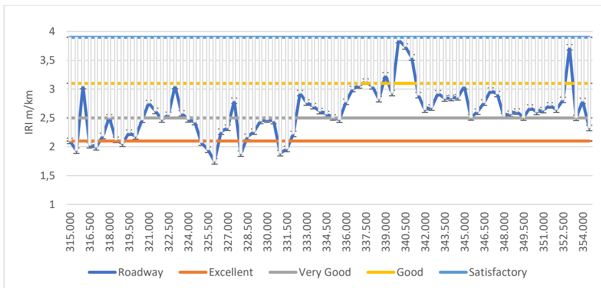
Fig. 3. Smoothness indicators of the cement-concrete pavement on the 315-355 km section of the A 380 highway
