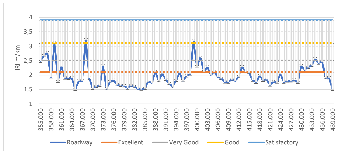
Fig. 4. Smoothness indicators of the cement-concrete pavement on the 355-440 km section of the A 380 highway
