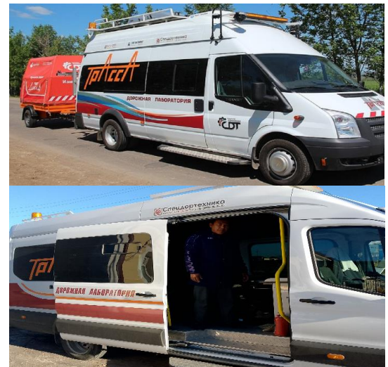
Fig. 1. "TRASSA" mobile road laboratory vehicle
