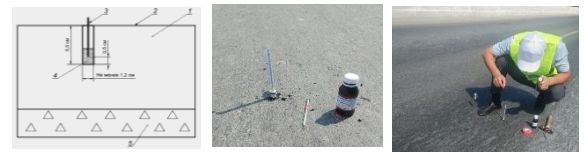
Fig. 2. Scheme for measuring the temperature of asphalt concrete:
