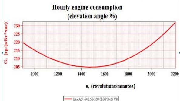
Figure 2. Graphical representation of the engine's hourly consumption at 0 percent height
