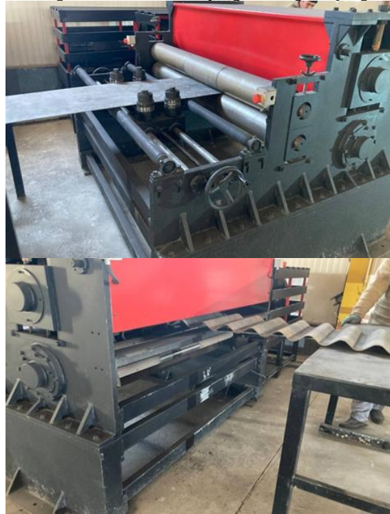
1-rasm. Qo'shtavr devorchasini gofrlash jarayoni (Samarqand)
