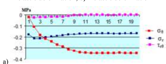
Fig. 8. Parcelling of tangential, radial and tangential stresses around the excavation at \theta=0^\circ and H=15 m: a) elastic deformation, b) inelastic deformation
