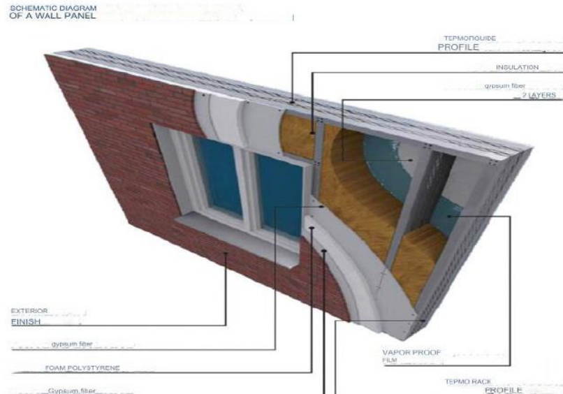
Figure 1. Diagram of a frame-sheathing wall
