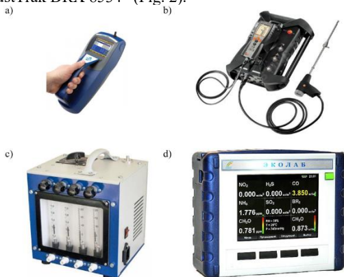
Fig. 2. Gas analyzers of the Center for Specialized Analytical Control: a) “DustTrak DRX 8534”; b) "Testo 350"; c) Aspirator; d) ECOLAB
